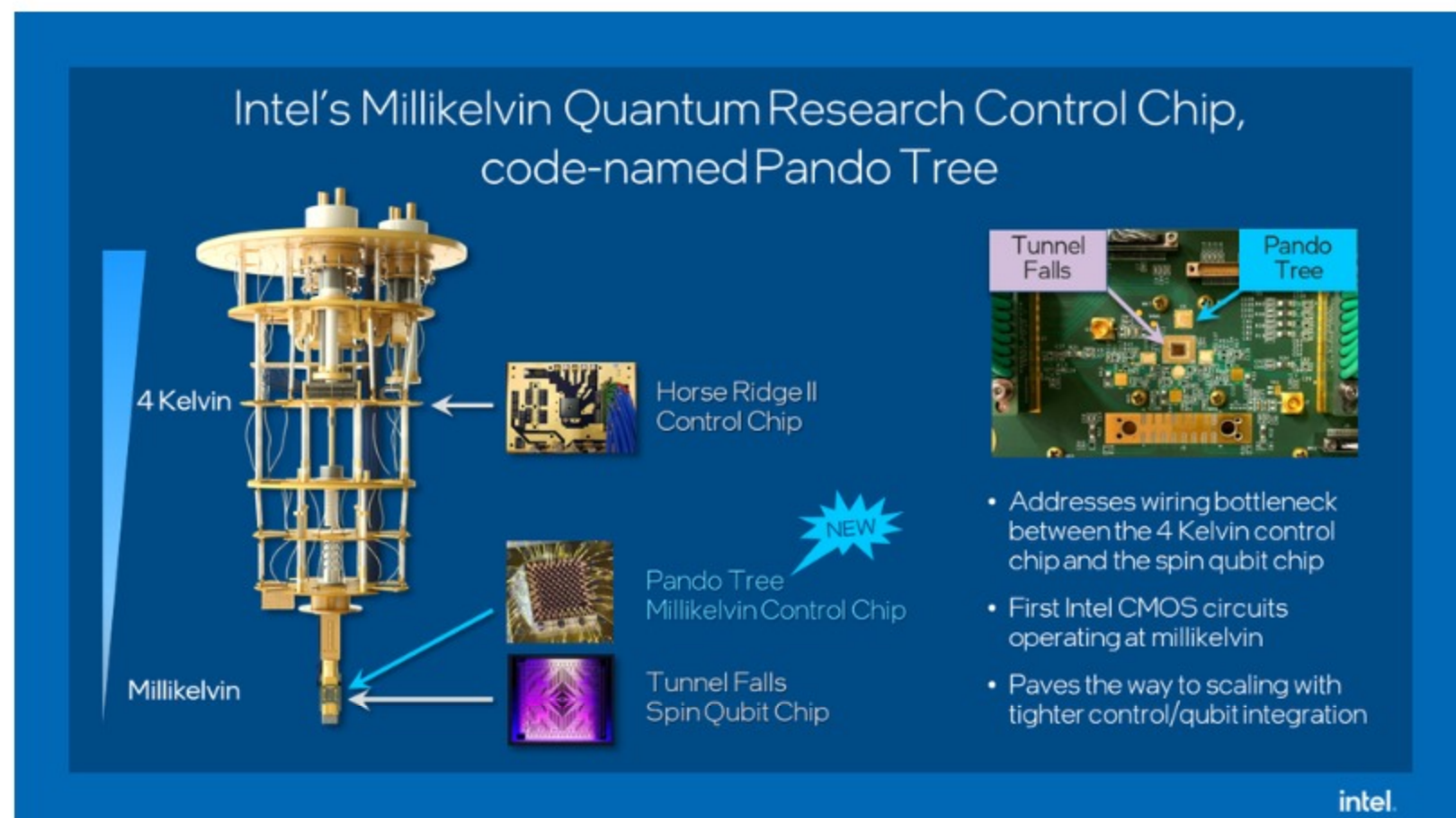
Figure 1. Intel's millikelvin control chip, Pando Tree, is closer to the spin qubit chip.
